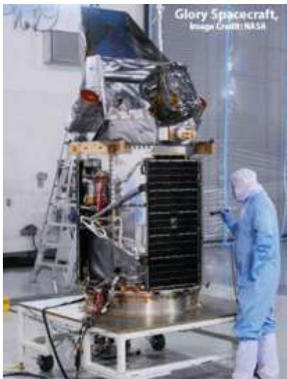
Above: The Glory spacecraft at the launch site during final checkout and processing. Photo credit: NASA.
